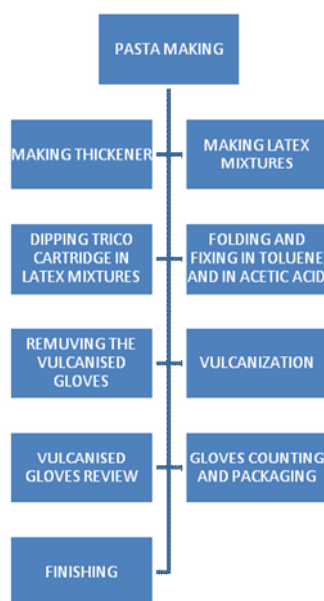
Figure 2. Schematic representation of the technological process of production of protective gloves. [4]
