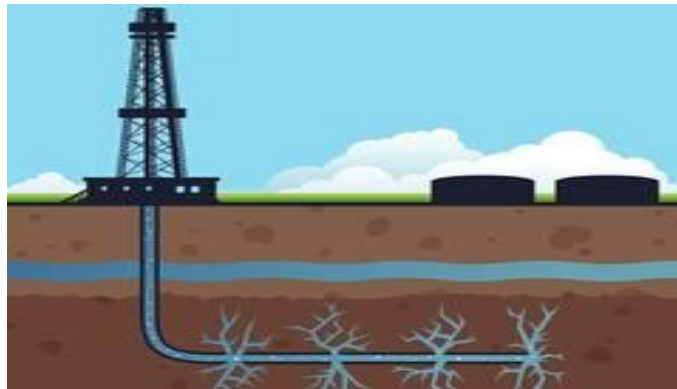
Figure 2. Scheme hydraulic fracturing method for shale gas
