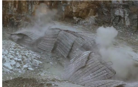
Figure 7 Initiation of blasting charges covered with blasting mats in quarry rock blasting [14]
