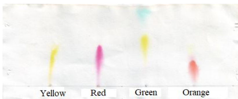
Figure 2 Chromatogram of colours isolated from a candy sample
