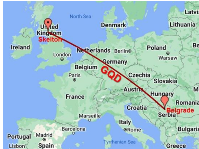
Figure 2 Great Circle Path (red) of VLF radio signal GQD/22.1 kHz, transmitted from Skelton (UK) and registered in Belgrade (Serbia)
